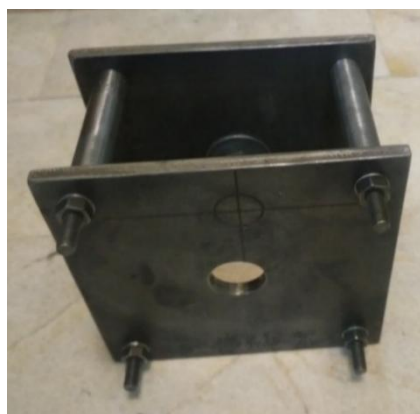
Fig. 5. View of the holding fixture in the impact test facility and how to mark the hit point before installation of the sample
